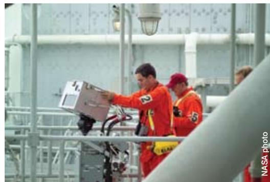
This upgrade to a prototype system uses near-infrared wavelengths to detect ice on the shuttle’s external tank. The new system is lighter and smaller as well as more reliable and user friendly. A joint effort between Kennedy, the U.S. Army Tank Automotive Research, Development, and Engineering Center, and MDA Corporation, the camera system is slated to be used during the February 2010 shuttle launch.
