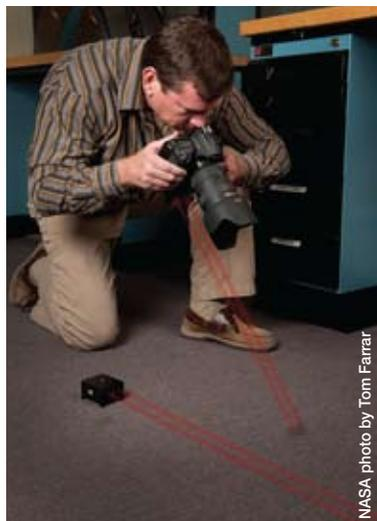
Starting with an idea from two shuttle engineers, Youngquist built a prototype device using laser beams to provide scaling information. He then worked with others to develop software that computed the distance scale.
